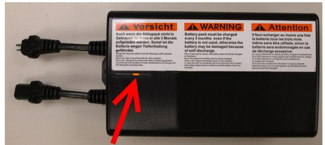
3. When the light changes to green, charging is complete. Disconnect the power supply unit from the main electrical source and then disconnect the transformer from the charger.
