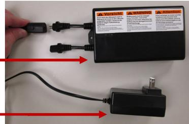
2. The red light on the battery will flash while the battery is charging. (It may take several seconds after connecting to power source.)
